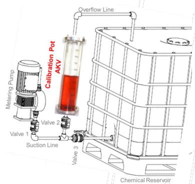
To check dosing pump rate isolate the chemical inside the calibration pot, leave valve #3 close and valve #2 fully open. Start the pump for one minute operation and observe the number of marks on the scale the fluid passed. This value provides actual metering pump performance per minute for particular chemical its concentration and discharge conditions.
